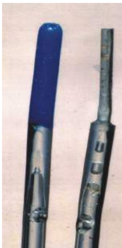
● Fig. 9.1 Intact Braun flexible tip catheter on the left, with absent tip on the right, following removal from patient.
